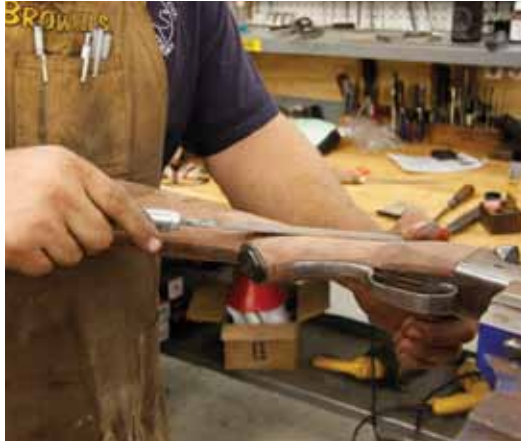
Shaping of stock around the pistol grip.
